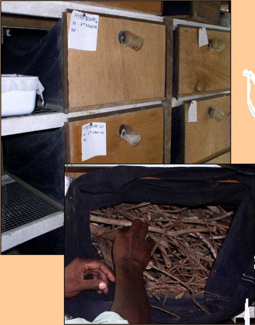
Extractors are used to collect bark beetles emerging from the timber samples.
